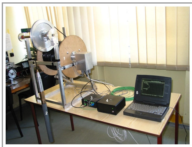
Fig. 3. General view of measuring system: 1 – revolving drum with optical fibre, 2 – underground receiver, 3 – processing block, 4 – ground receiver, 5 – computer.
