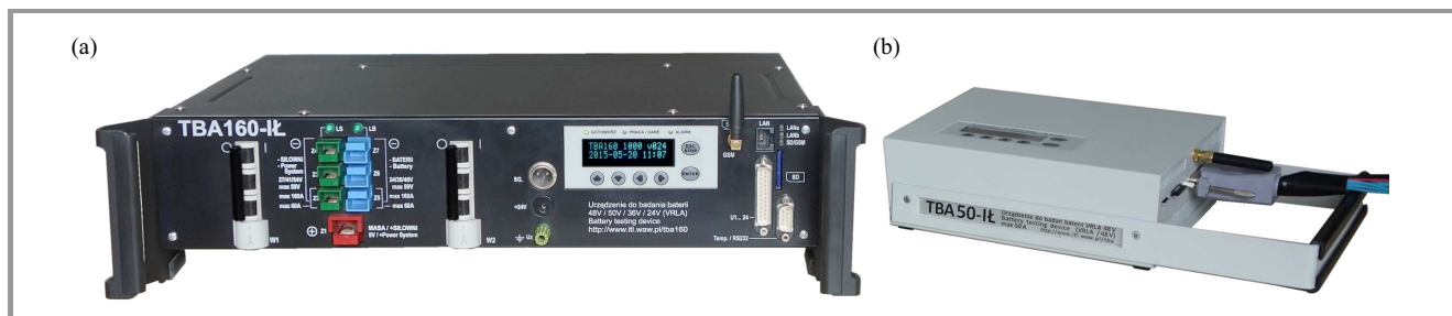
Fig. 3. Stand-alone battery ATE: (a) up to 160 A and (b) up to 50 A.
