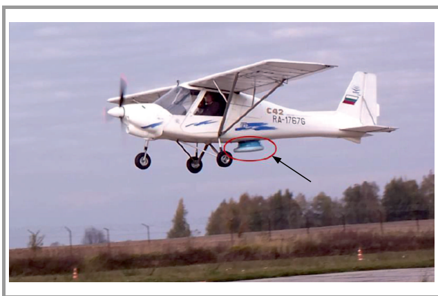
Fig. 1. IKARUS C42 plane with aviation-grade RVS, during testing.
