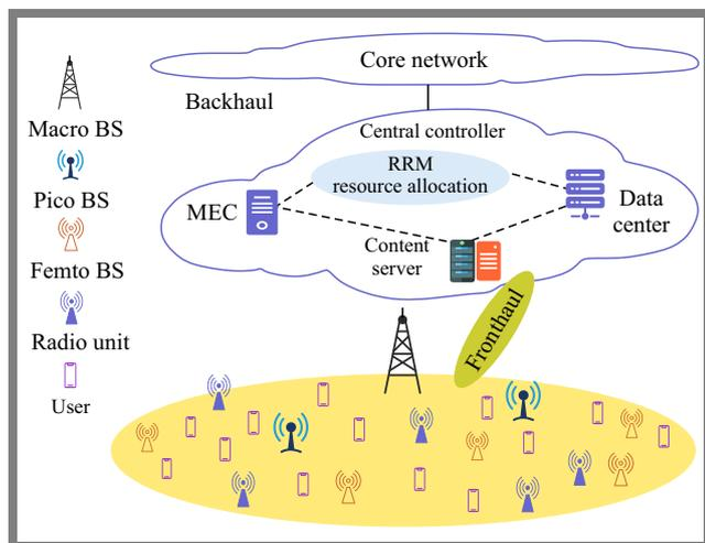
Fig. 3. RRM technique in a cell-less architecture.
