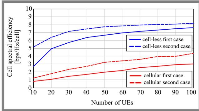
Fig. 7. CSE for different UEs for both interference cases.
