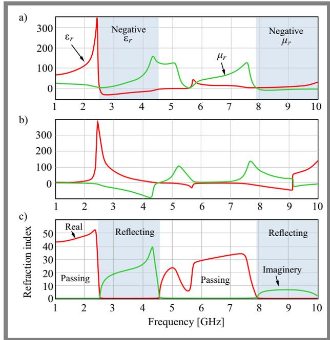
**Fig. 4.** Constitutive parameters ( $\epsilon_r$ ,  $\mu_r$ ): a) real, b) imaginary component, and c) refractive index.
