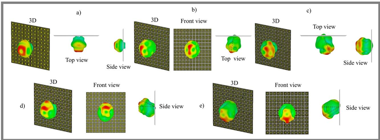
**Fig. 10.** Radiation pattern of the proposed structure in the case of: a) all diodes in on state, b) group A being in the on state, c) group B being in the on state, d) group C being in the on state, and e) group D being in the on state.
