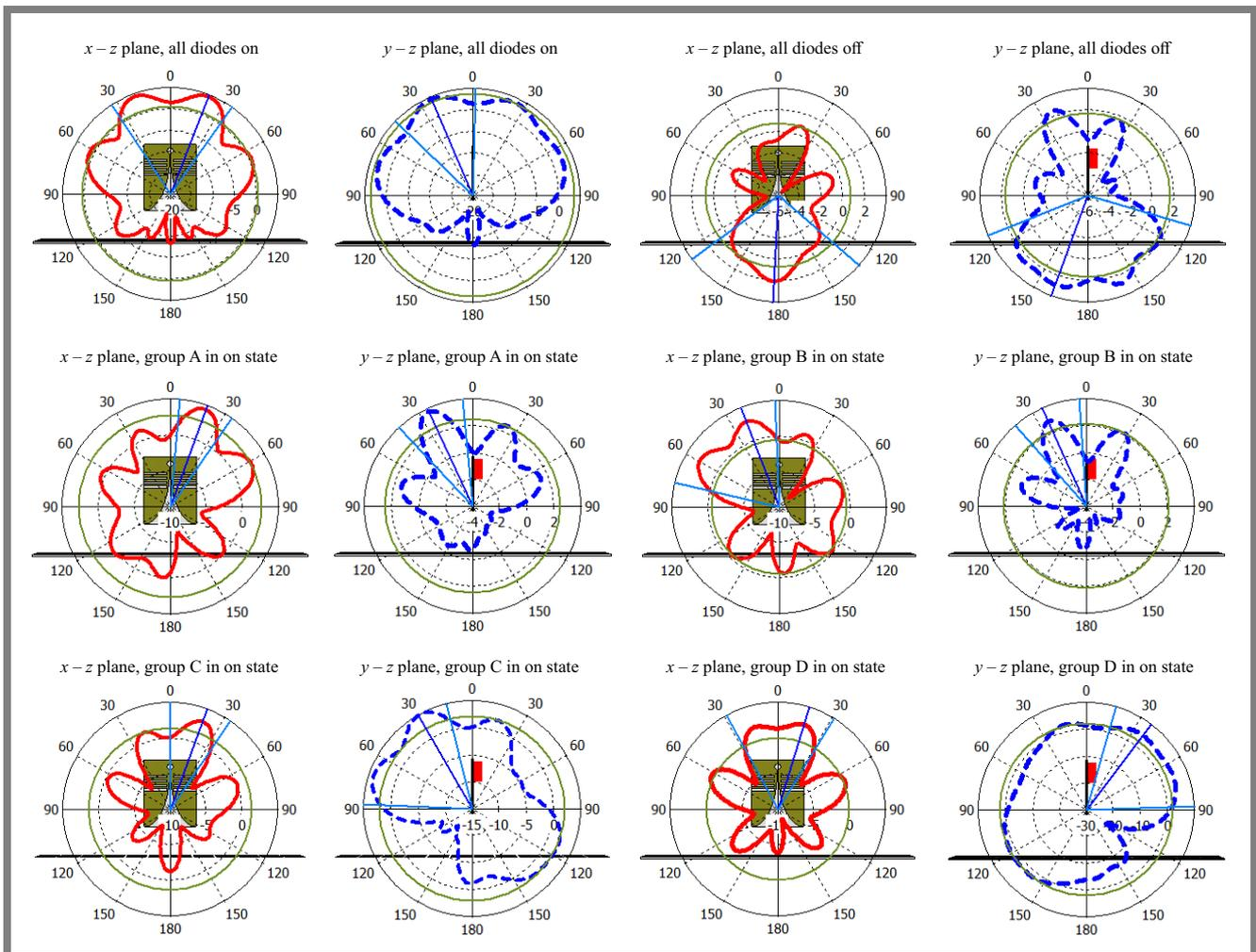
**Fig. 11.** 2D projection of radiation patterns of the proposed structure for different states of the diodes.
