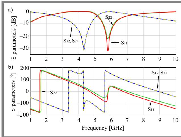
**Fig. 3.** S parameters of the unit cell: a) magnitude and b) phase.
