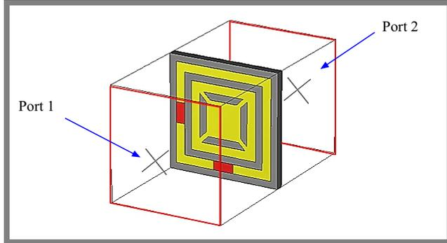
**Fig. 2.** Fictual waveguide with port excitation entries and boundary conditions settings.
