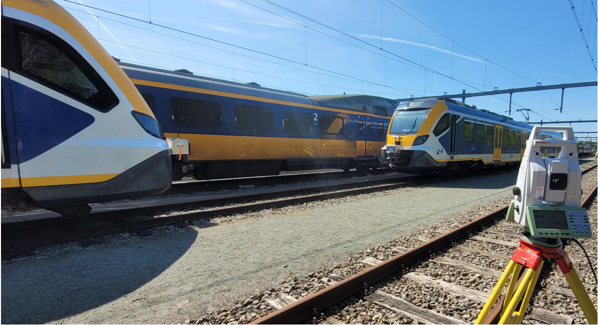
Figure 2.5: T2T Communication and ranging tests using IEEE 802.15.4.
