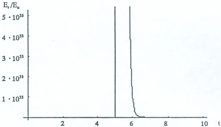
Fig. 6. The pulse reflected from the half-space with time-splashing conductivity (arbitrary units) t - normalised time
