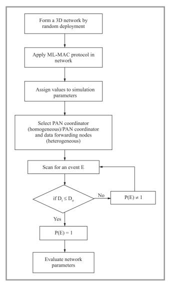
Fig. 3. Flowchart of steps during network simulation.
