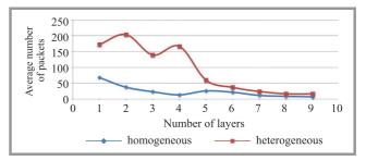
Fig. 5. Comparison of packets dropped for both networks.
