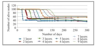
Fig. 9. Life chart of sensor nodes for homogeneous WSN.
