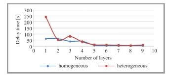
Fig. 6. Comparison of end-to-end delay for two networks.
