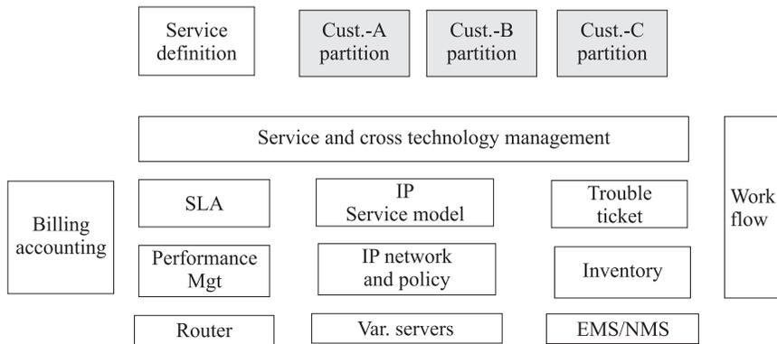
*Fig. 10. OSS-architecture optimized for services*
