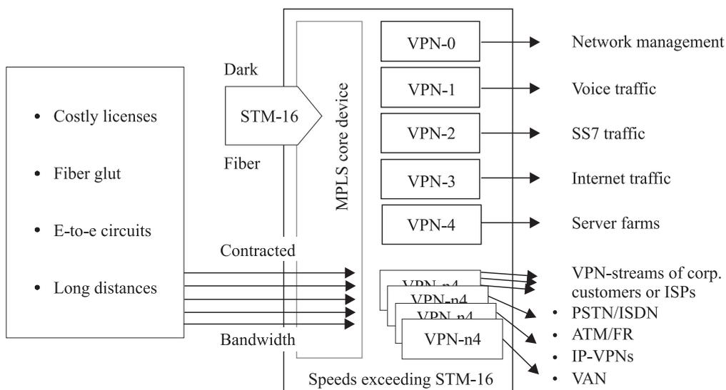
Fig. 5. MPLS – mapping VPNs to traffic streams
